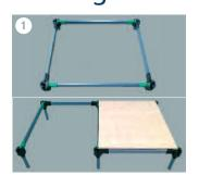
Using 150mm legs create the first row by assembling rails as per for a standard stage. Once the frame is complete add a single deck panel to 'Square' the unit. Then continue to build until the first row is completed.
